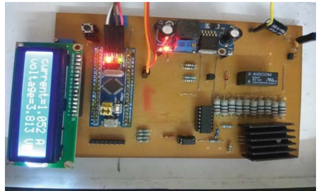
Fig. 1. Load circuit for cell characterisation.
